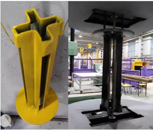
Fig. 7 On the left the jaws after painting in yellow, on the right the bar is fixed in the jaws in the testing machine before painting the jaws.
