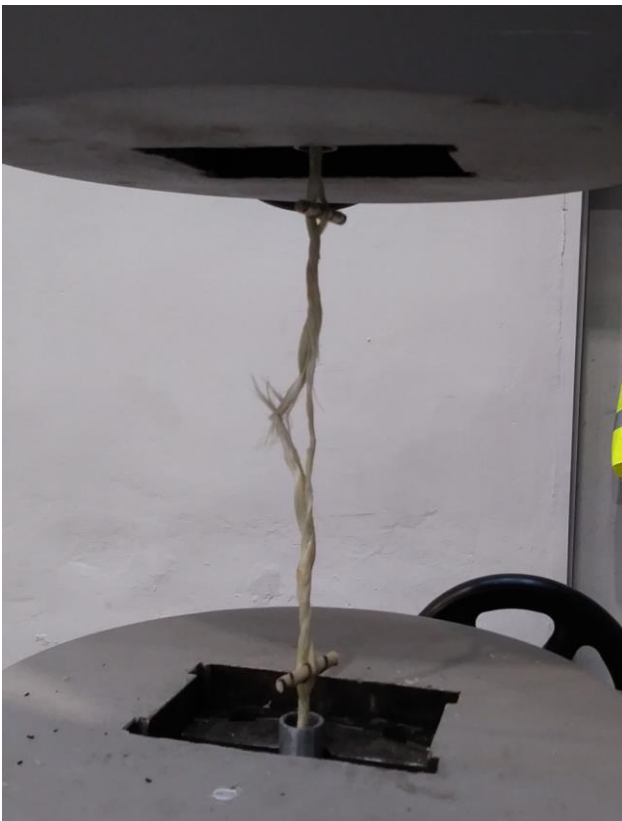
Fig. 4 Rod in a testing machine after breaking.
